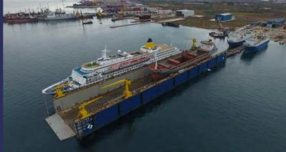
Floating Dock: 260m x 45m Dock Crane: 15tn x 22m/ 5tn x 15m Pier: 170m x 12m Harbor Crane: 15tn x 22m Slipway 1: 150m x 35m Crane: 2 x 50tn Slipway 2: 120m x 35m Crane: 2 x 50tn
